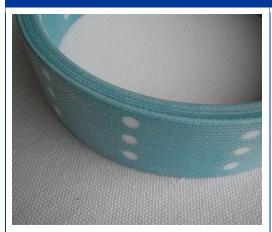
AS RS41 bearing materials is reinforced weave polymer material special developed for high loads and smooth running with lowest possible friction. The material contains an ideal concentration of polymer which gives the very good result in areas were reduced friction and wear is required. AS RS41 is also provided with thermoplastic dimples for further reduction of friction.
